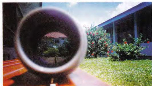
**6-P3** Pengurangan keamatan cahaya yang melalui kedua-dua Polaroid berbanding cahaya sekitar / Notice the reduced intensity of light through the two polaroids as compared with the background
